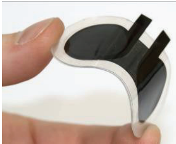
Figure 7: Flexible printed thin-film-battery consisting of two cells
