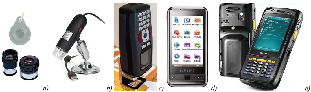
Figure 15: Used optics and scanning devices: Jelly Lens TM Close-Up and PEAK magnifier loupes (a), digital microscope dnt DigiMicro 1.3 (b), code scanning device Omnitron MAH300 (c), camera phone Samsung Omnia 900i with Windows Mobile OS (d) and the personal digital assistant (PDA) Pidion BIP-6000
