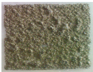
Fig. 9: poor print quality of the first pastes
