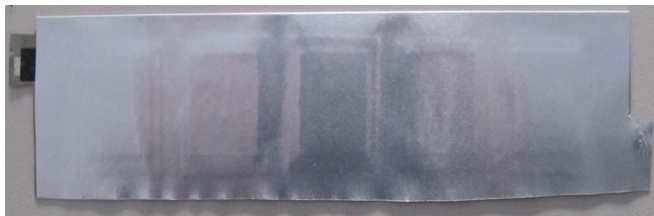
Fig. 16: Five printed zinc-manganese dioxide cells in series connection
