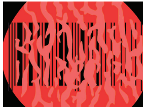
Fig. 1: "Collapse" into pieces of bar-code applied to a contoured surface of the swollen rubber
