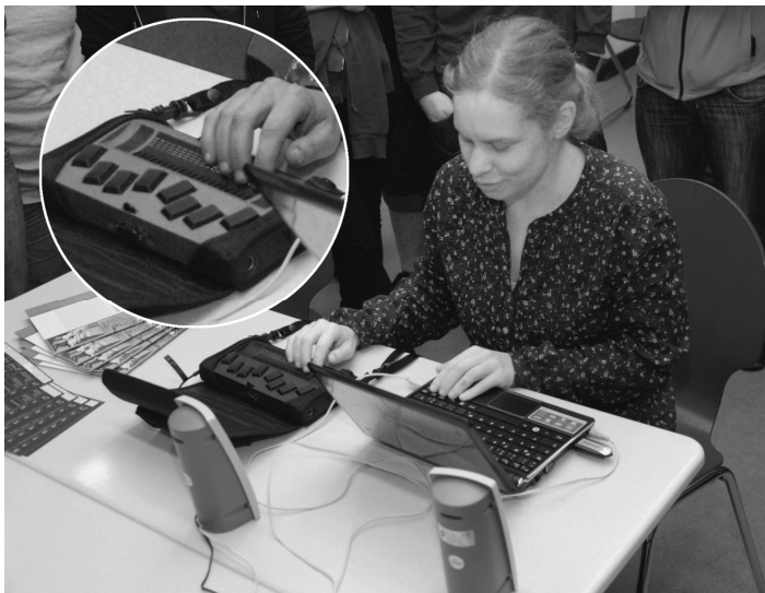
Figure 1: User interaction with keyboard (right) and refreshable Braille display (left)
