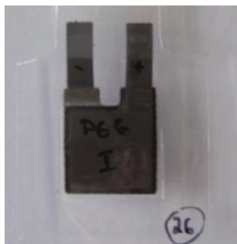
Fig. 7: The first prototype of secondary cell (in PET) [5]
