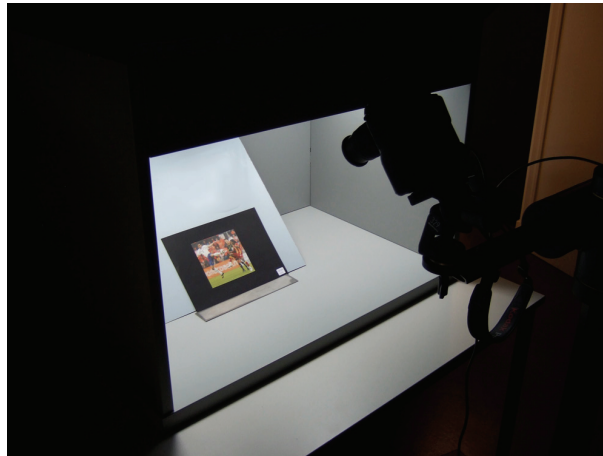
Figure 1: Camera setup for making digital photographs of the printed pictures
