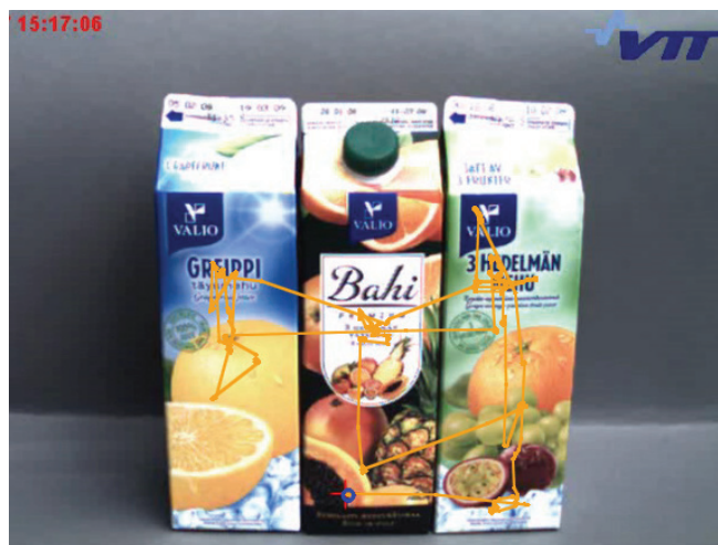
Figure 2: Scan path for an observer viewing the real packages. Frame capture from a video showing the gaze location overlaid on the scene video. The point and crosshair cursor indicates the current gaze location. The trailing line depicts the gaze path during the last 10 seconds
