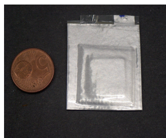
Fig. 11: Battery concept in stacked-type
