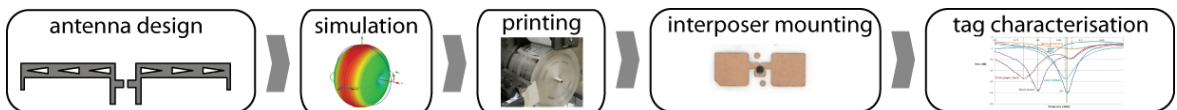
Figure 6: Workflow concept to manufacture a package with included RFID functionality: antenna design, simulation, conductive ink printing, interposer mounting of Si microelectronics, tag characterization (from left to right). For this procedure, an adaptation in the software workflow concept is required.
