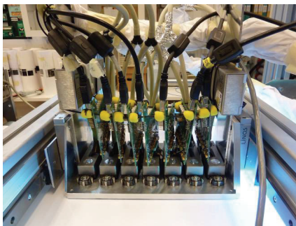
Figure 3: The seven print head assembly with conical adjustment screws. The green printed circuit boards are the head driver cards and the two boxes over the heads at the ends, contain ink temperature and meniscus pressure sensors
