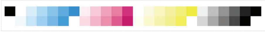
Figure 2: Simple ramp test target that used simple C, M, Y and K, 10 step ramps from 10% to 100% at 10% intervals
