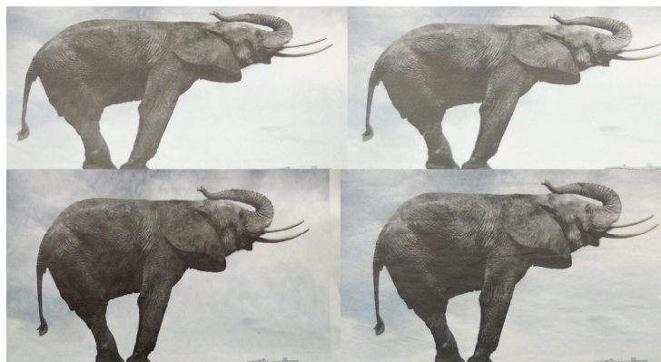
Figure 6: Differences in perceived dynamic range as a result of ink-gloss. The pictures on the first row are top-lighted and recording under 45°. The pictures on the second row are tilted under 45° (newspaper are often read in this way)
