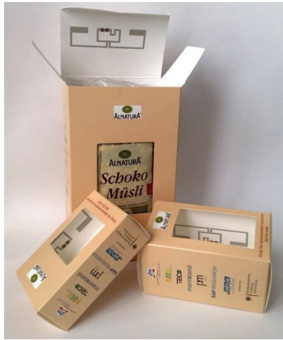
Figure 5: Packages with RFID functionality based on printed RFID antennae
