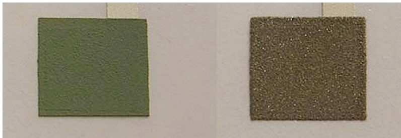
Fig. 6: Electrode layers printed several times with intermediate drying cathode (left) and anode (right)
