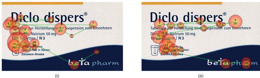
Figure 4: Sample scan paths from pharmaceutical packaging design analysis. Each circle visualizes a fixation of the viewer. The numbers in the upper half of the circle specify the order in which the fixations were made, the number in the lower half and the size of the circles visualize gaze duration
