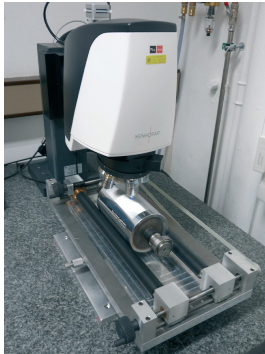
Figure 1: Measurement setup: Confocal microscope (Sensofar Plu Neox) equipped with an adjustable stage for the gravure cylinders
