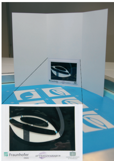
Figure 4: Integration of the smart system to a card demonstrator; including a zinc-manganese battery, a push-button and assembled components
