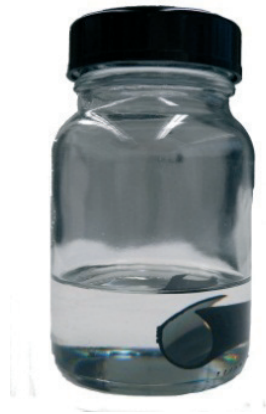
Figure 2: Test sample in a glass vessel at static solvent resistance test
