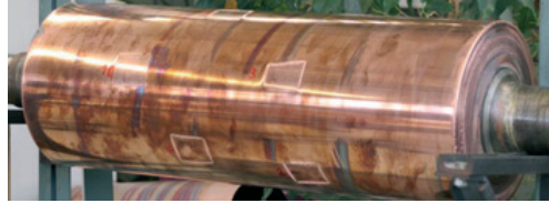
Figure 5: Copper cylinder with patches of reduced layer thickness
