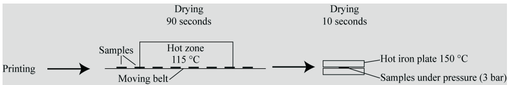
Figure 3: Schematic representation of two stages combined drying process
