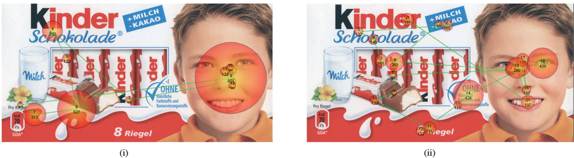
Figure 5: Sample scan paths from chocolate box design analysis. Each circle visualizes a fixation of the viewer. The numbers in the upper half of the circle specify the order in which the fixations were made, the number in the lower half and the size of the circles visualize gaze duration
