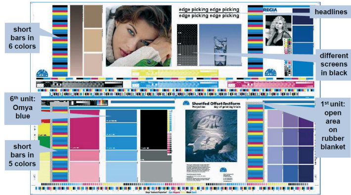
Figure 1: Layout developed for evaluation of edge picking in commercial offset printing trials (Dahlvik et al., 2011)
