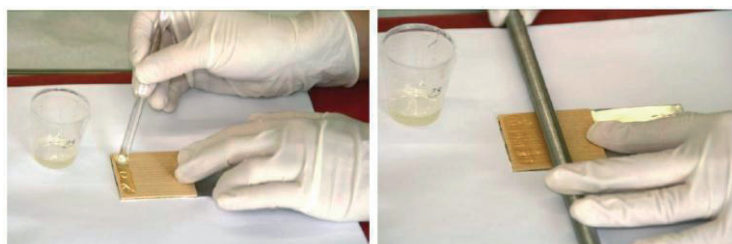
Figure 8: Application of the clear varnish on spruce veneer by manual roller coating
