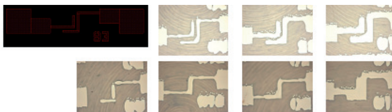
Figure 7: Example of structures used to electrically obtain metal layer line separation design rule with the design drawing (top-left) and some right (top) and wrong (bottom) of the fabricated samples
