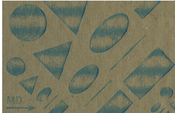
Figure 2: Detail of printed sample with obvious washboarding. The alignment of the flute is indicated by the arrow
