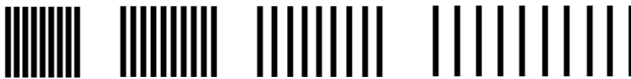
Figure 6: Example of structures used to optically obtain single layer line separation design rule
