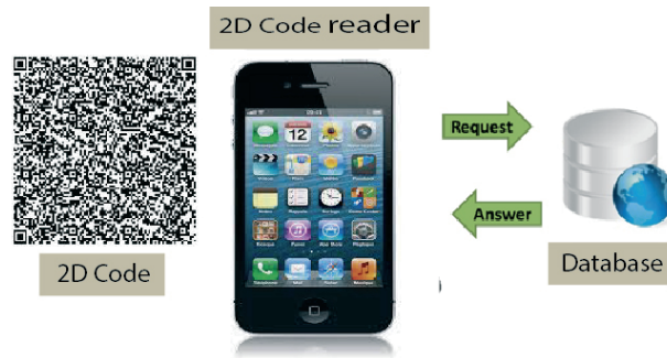
Figure 1: Principle scheme of the use a 2D code for authentication and traceability
