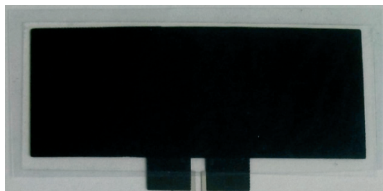
Figure 4: 3 V battery delivering 1 mA of current
