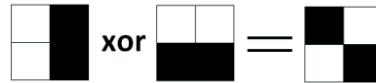
Figure 5: xor treatment on a simple example of 4 pixels (first square represents the printed sample, the second one, the numeric file and in the last one, the black dots symbolize the similar pixels)
