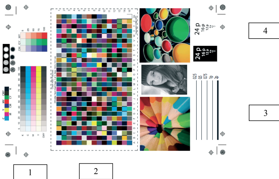
Figure 1: Test image 1 - color control patches of CMYK and RGB colours, 2 - 400 patch test chart for gamut sampling, 3 - different lines, 4 - letters in different sizes
