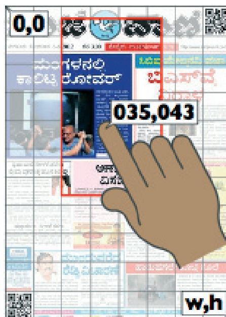
Figure 3: The AudioCanvas coordinate system. Touch point coordinates on the user's photo of an object are calculated based on the distance between and relative sizes of the two QR codes detected on the item. The resolution of the coordinate grid is high enough to allow zooming in to the image and very precise selections, if necessary. Touching a point causes a six-digit DTMF-encoded request for the relevant audio to be sent to the voice site. The audio is played over the phone line in response. The grid is not visible during usage
