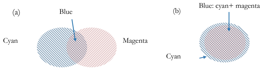
Figure 1: Dot area coverage for: (a) Demichel method; (b) Dot-on-dot screen
