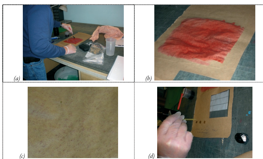
Figure 1: Illustration of methodology to describe barrier properties. (a) show the application of liquid on the barrier surface, (b) a barrier surface after liquid application, (c) the backside of a barrier printed substrates after ten minutes with stains that has penetrated through the substrate, and (d) illustration of oil drop test with conventional olive oil
