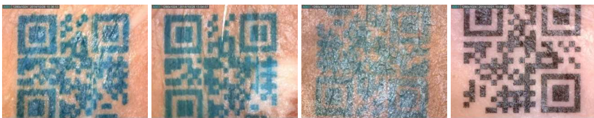
Figure 3. Comparison of the inks on ham slices: from left Edible ink 1, 2 and 3, and Solvent based ink. Cell size is 1.00 mm.
