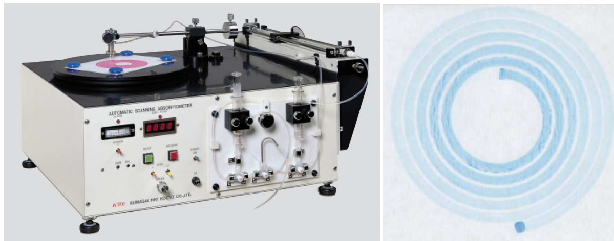
Figure 1: Left: ASA instrument. Right: Spiral stain from ASA measurement, the inner & outer circles correspond to longer and shorter contact time, respectively.
