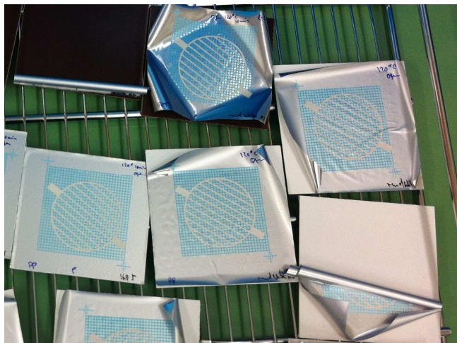
Figure 2: Effect of oven curing on the dimensional stability of the substrate. When adhesion was too weak, the samples pulled off and curled.
