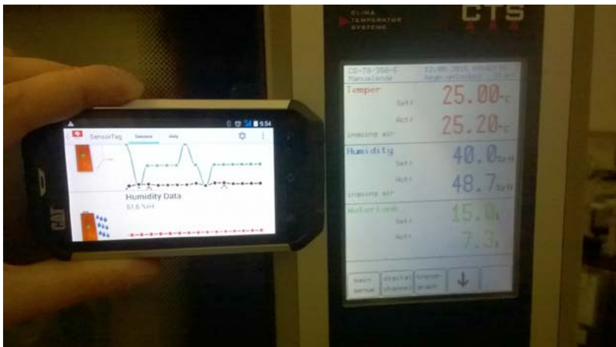
Figure 9: Data comparison of sensor tag, which is used as reference, and thermal couple imbedded in CTS
