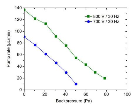
Proof-of-concept: First transparent, inkjet-printed micropump actuator Low backpressure due to passive valves → Modify valve concept
