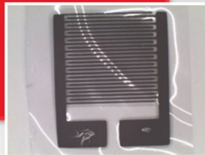
NFC based sensor before/after cycling in humidity chamber
