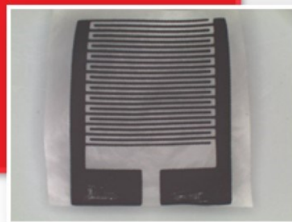
NFC based sensor before/after cycling in humidity chamber
