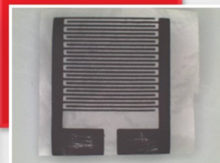
NFC based sensor before/after cycling in humidity chamber
