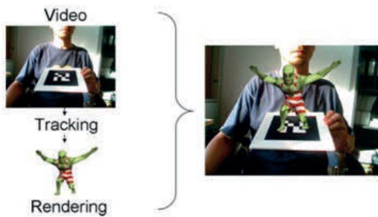
Figure 1: Data flow in a common augmented reality system (Kalkofen, et al., 2011)
