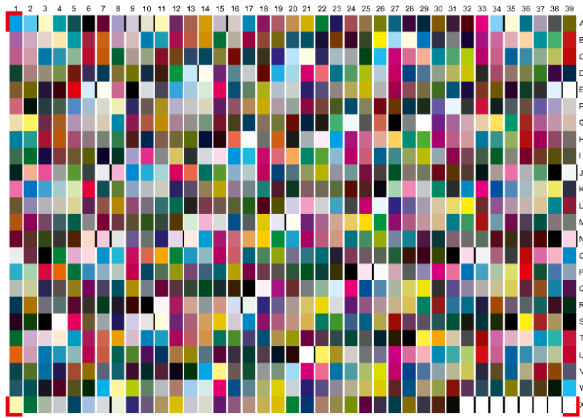
Figure 2: EFI profiling chart IT8 i110 (originates from software EFI Fiery XF 6), 936 randomised patches in 39 columns and 24 rows, patch size 7 mm × 9 mm, printed in 32 cm × 23 cm
