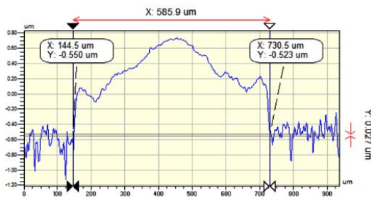
Figure 4: Cross section and width of the printed fine line measured by white light interferometry
