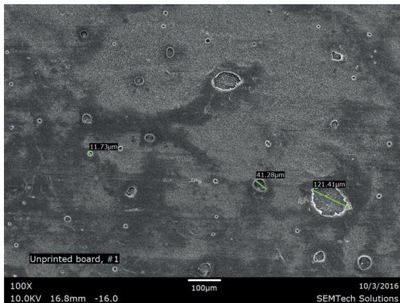
Figure 1: SEM image of pitted surface of curtain coated board
