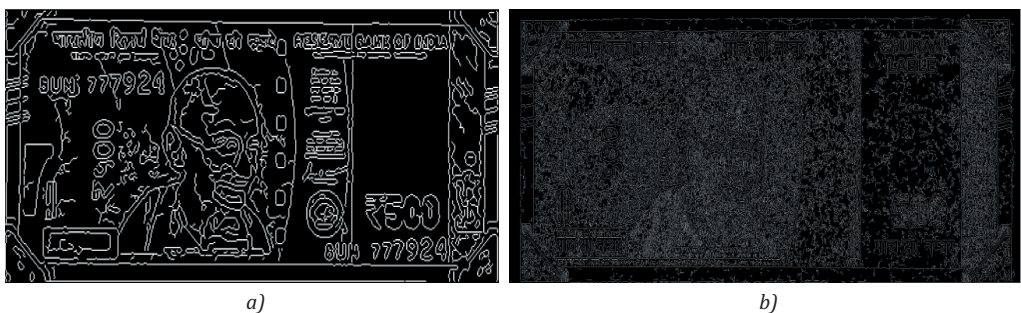
Figure 9: Canny edge detection of real and dummy currency note: (a) real, and (b) dummy
