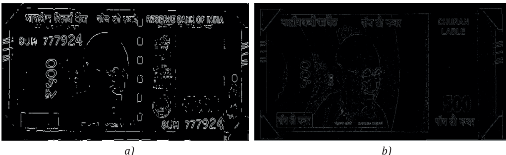
Figure 10: Sobel edge detection of real and dummy currency note: (a) real, and (b) dummy
