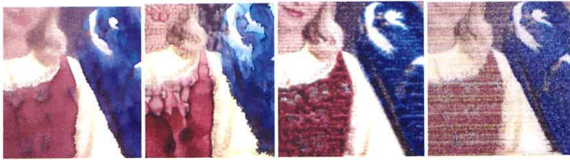
Figure 7: Printed samples (from left to right) on glossy and matt side of Ensocup with solvent-based ink (SB-M1), on coated side of Ensocoat with solvent-based (SB-M1) and with oil-based ink (OB-M7)
