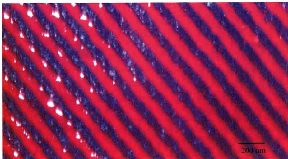
Figure 8: Microphoto of the anilox roller surface (55x magnified). The cell walls appear dark, while the cells appear brighter. Water on the surface is visible as white areas. (This photo shows a section of the anilox roller on the border between solid area and non-printing area of the printing forme. The solid area is located in the left part of the photo.)
