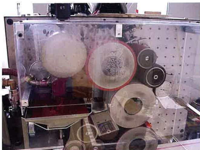
Figure 9: Humidity condensation on the insides of the Plexiglas windows. It indicates the transgression of the dew point in the steamy areas
