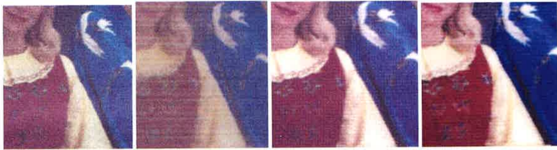
Figure 8: Printed samples (from left to right) on cloth with solvent-based (SB-M1) and oil-based (OB-M7) ink, on polyester with solvent-based ink (SB-M1) and on vinyl with solvent-based ink (SB-M1)
