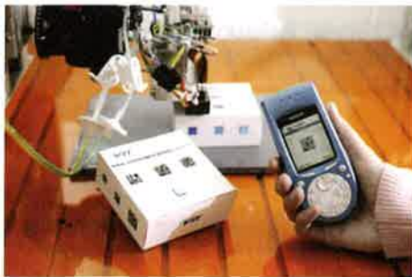
Figure 8: Example of reading a two-dimensional bar code from a package with a camera phone
