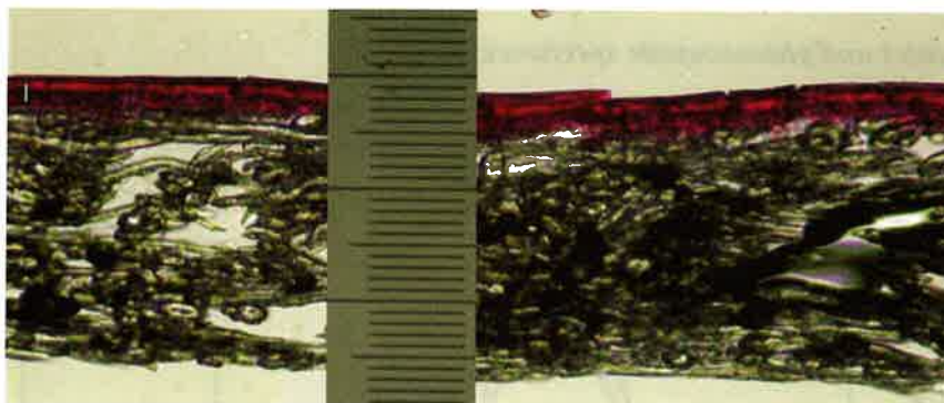
Figure 8: The microtome cross section analysis of Z sample with added micrometer measuring tool
