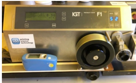
Figure 2: Laboratory flexo printing machine IGT F1 printability tester and micro-tri-gloss (in blue in the bottom left) on a printed substrate
