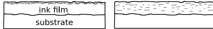
Figure 1: Distribution of leafing (left) and non-leafing (right) aluminum pigments in ink (Weber, Spiehl and Dörsam, 2022)
