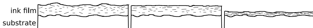
Figure 12: Schematic of ink levelling of metallic inks on a rough substrate with a relatively high porosity and roughness
