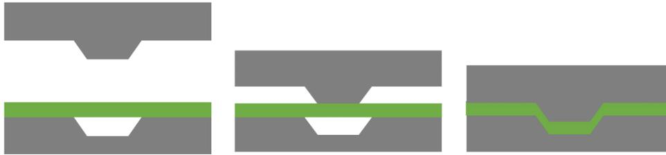
Figure 6: Schematic representation of the embossing process (flat embossing, relief embossing) – left side: wide spacing of the embossing tools, no material contact; middle: first material contact without shaping; right: material shaping, embossing tools move into each other
