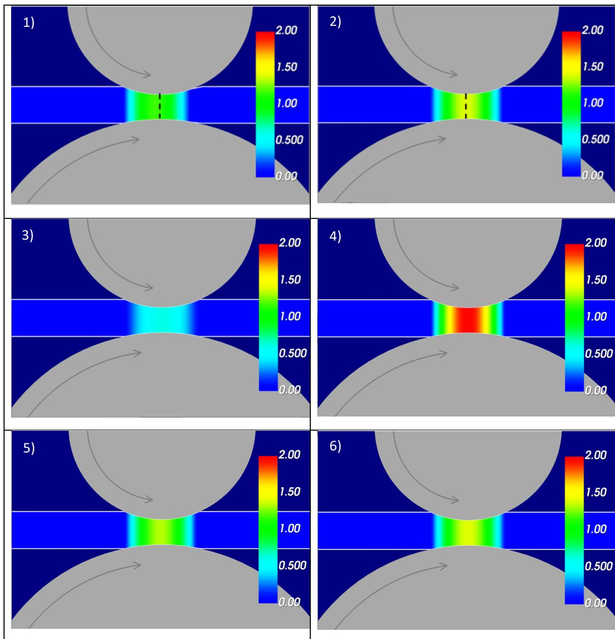
Figure 3: Three pairs of examples of nip pressure distribution; the material properties and the printing speed used in the simulations are given in Table 1, the dashed lines in images 1 and 2 stand for the position of the nip center
