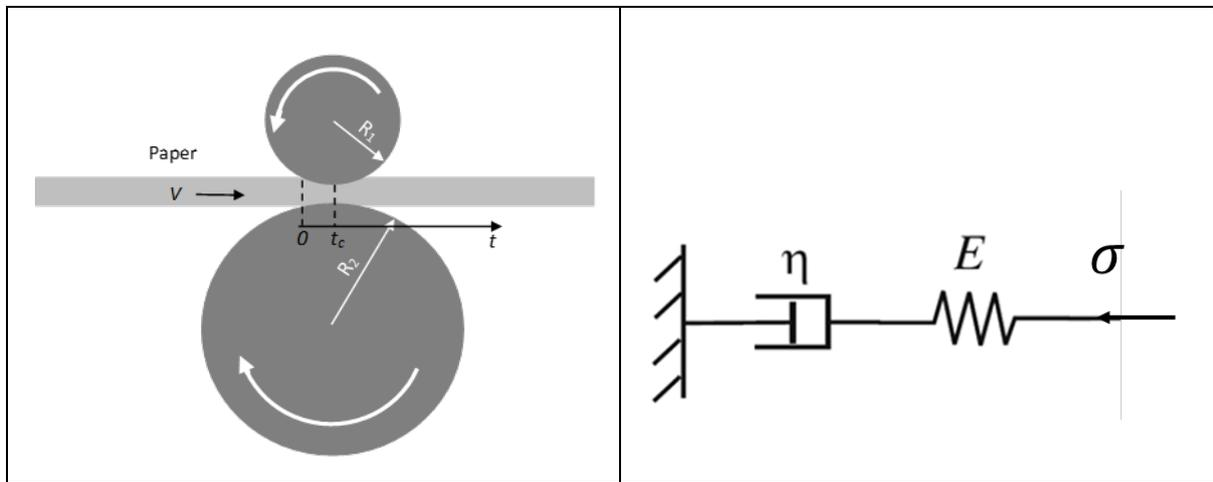
Figure 1: Illustration of the rolling nip between two rigid cylinders (left),  $t_c$  is the time duration from entering the nip to reaching the nip center; and the material model of the paper (right)
