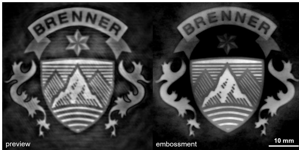
Figure 9: Direct comparison of the estimated heightmap of the embossing preview and an actual 3D scanned embossment in cotton paper with a grammage of 450 g/m 2
