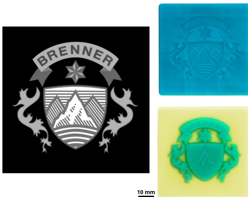
Figure 4: View of the 8-bit heightmap, on which the embossing tool to evaluate the plausibility of the embossing prediction is based (left) and an image of the embossing tool derived from it, consisting of a female die (top right) and a male die (bottom right)
