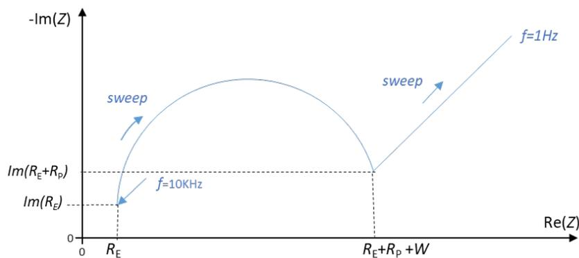
Figure 5: Idealized Nyquist plot of a printed battery
