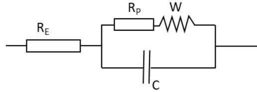
Figure 4: Equivalent circuit diagram
