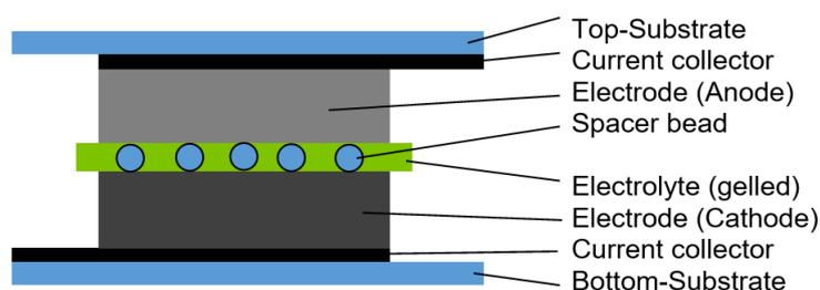
Figure 2: Side view of stack design with added spacers
