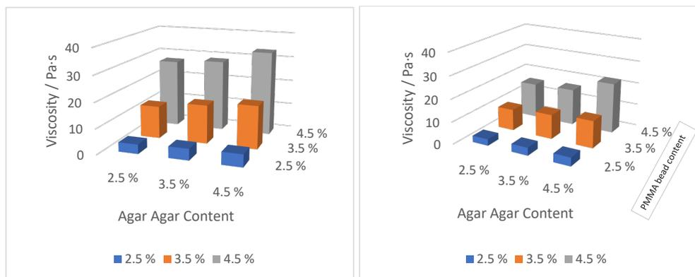
Figure 8: Viscosities of the different pastes left: at a shear rate of  $50 \text{ s}^{-1}$  and right at  $100 \text{ s}^{-1}$
