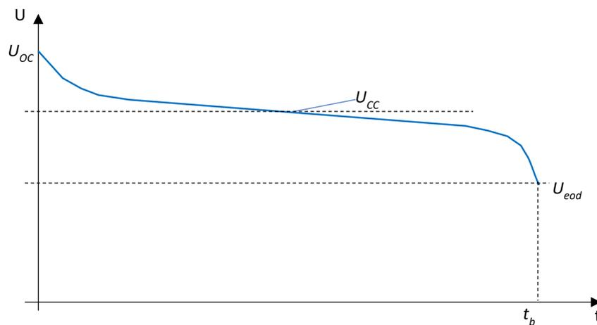
Figure 3: Typical CC-discharge curve of primary battery
