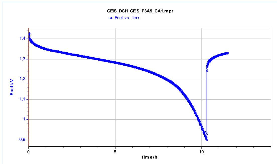
Figure 9: CC discharge curve of a battery with P3A5
