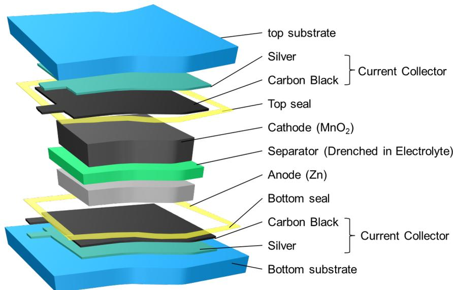
Figure 1: Explosion drawing of a printed battery in stack design
