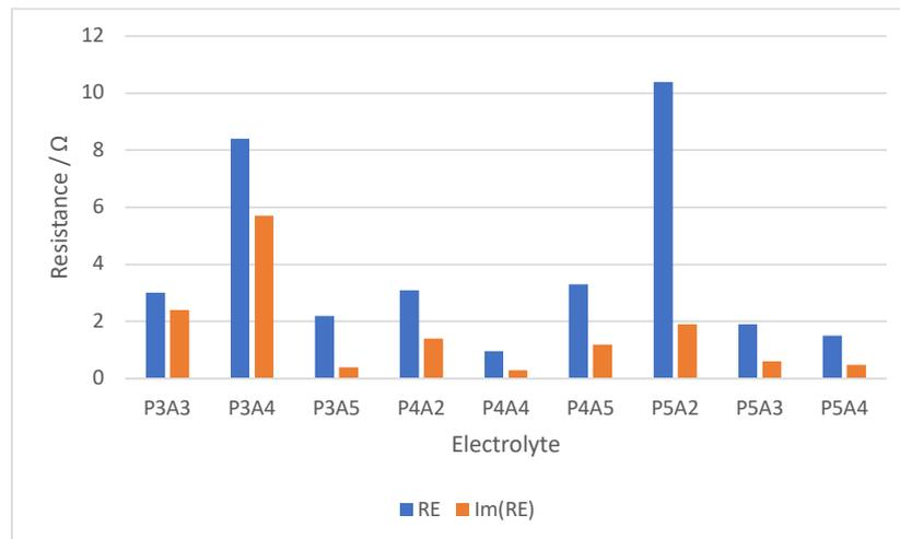
Figure 11: Inner resistances of assembled batteries (real and imaginary part of impedance)
