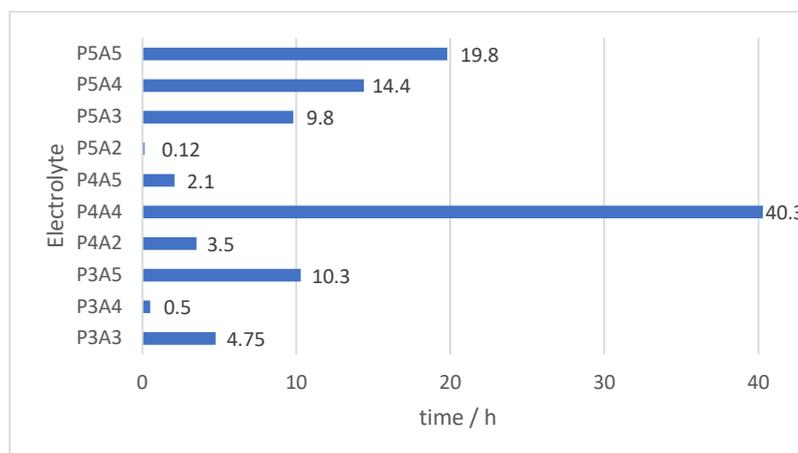
Figure 10: CC discharge results for batteries with different electrolytes
