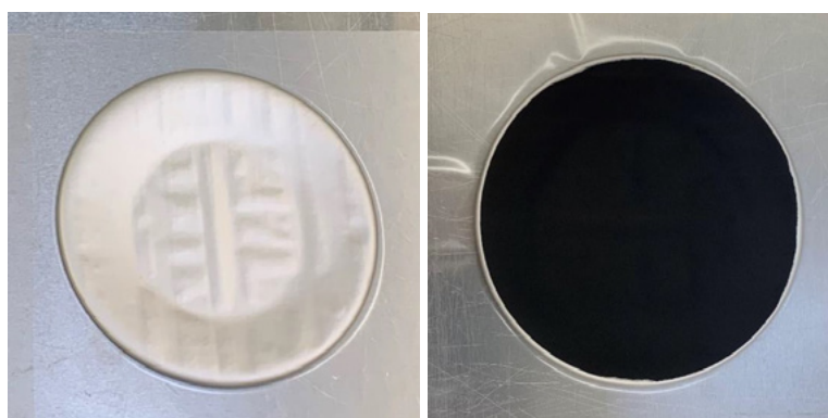
Figure 17: TPU substrate with printed current collectors on top; left: silver, right: silver plus carbon
