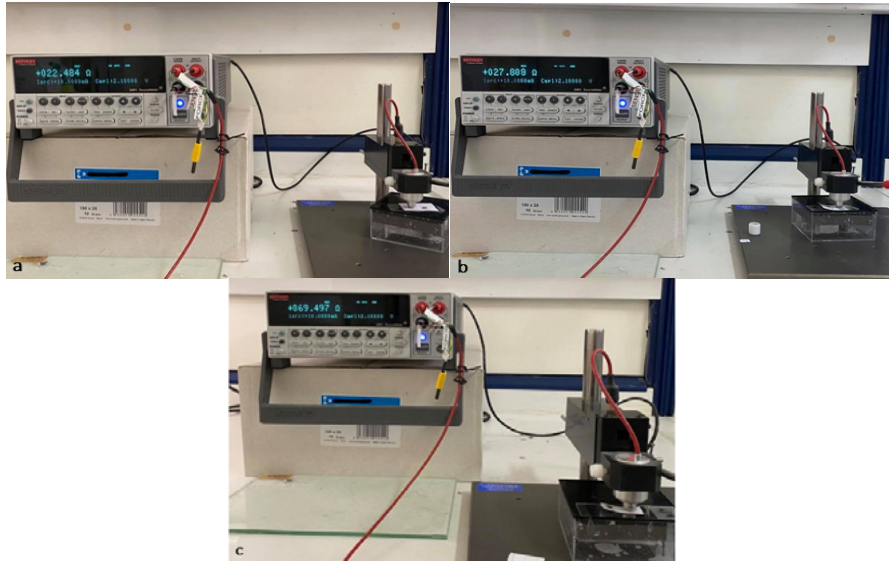
Figure 5: The R_s measurements of: (a) CB_{70} -rGO slurry, (b) CB_{70} -rGO(70/30) ink, and (c) CB_{70} -rGO(50/50) ink
