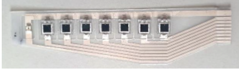
Figure 1: Printed flexible strip on PET with mounted SMDs for testing purposes
