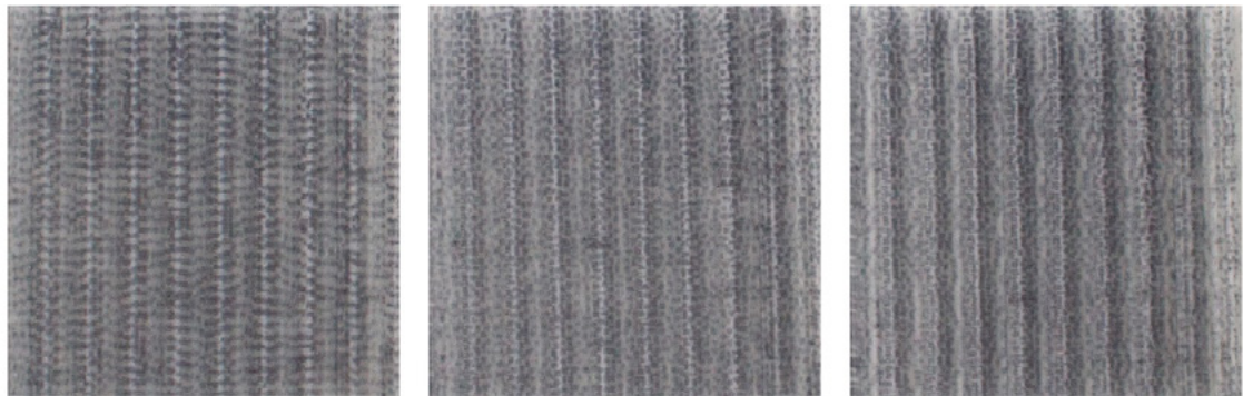
Figure 5: Print results, 3D views; filter parameters as \sigma_1 = 1.9 , \sigma_2 = 1 , left: parallel, middle: symmetric alignment, right: perpendicular halftones to the 3D structure variation
