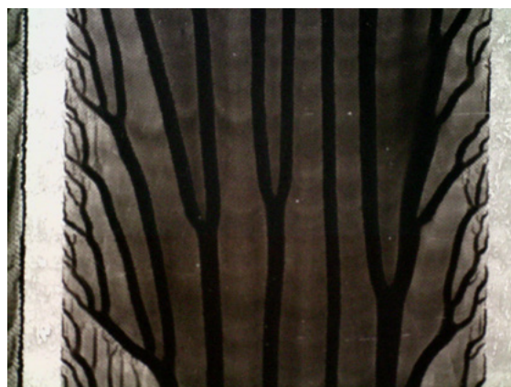
Figure 6: Representative detail of the gravure printed pattern with the CB 70 -rGO(50/50) ink for cell volume 9 \text{ml}\cdot\text{m}^{-2}
