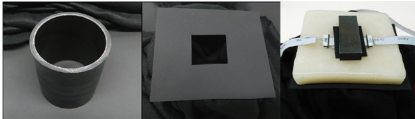
Figure 22: Measurement on a “black hole” to avoid influence of underlaying backing
