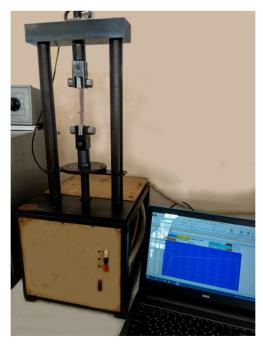
Figure 2: The equipment for testing the adhesive strength of laminates
