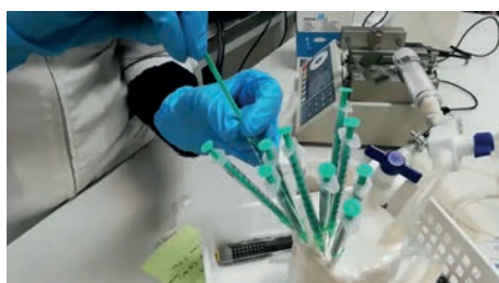
Figure 6: Taking care to isolate samples from contamination using a mechanical sealed pipette, transported in a film-sealed vessel
