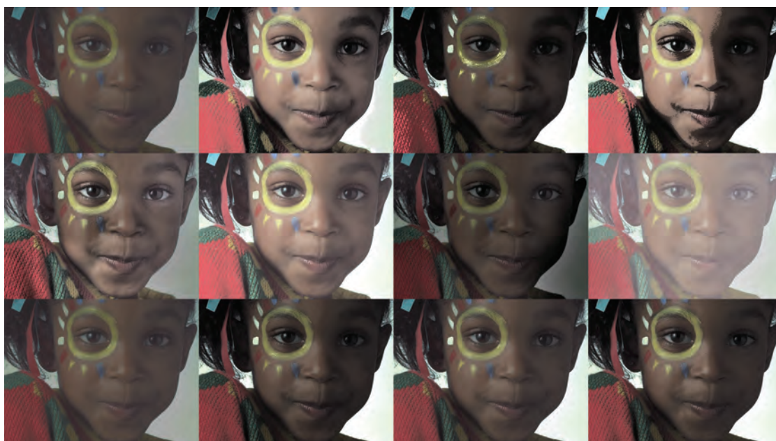
Figure 8: Results of different HE techniques for color test image ‘Girl’; (top row from left to right) original (input) image, GHE, BBHE, DSIHE, (middle row left to right) CLAHE, AGCWD, AMSR, LLIEA, (bottom row left to right) DFHE, GAHE, ABCHE, and presented HEBCO
