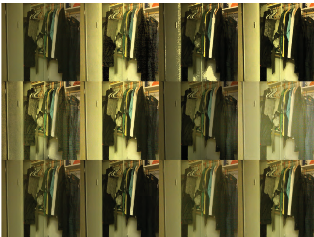
Figure 11: Results of different HE techniques for color test image from LIVE database; (top row from left to right) original (input) image, GHE, BBHE, DSIHE, (middle row left to right) CLAHE, AGCWD, AMSR, LLIEA, (bottom row left to right) DFHE, GAHE, ABCHE, and presented HEBCO
