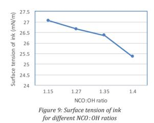
The surface tension values of ink formulated from different NCO: OH ratios were analyzed. Four PUDs based on four NCO: OH ratio, 1.15, 1.27, 1.35, and 1.4, have a constant molar ratio of polyester glycol and DMPA. When NCO: OH ratio is higher, the percentage of NCO increases while the amount of hydrophilic carboxyl group contents reduces. Reduced amount in ionic groups reduces polar group element of PUD; ultimately surface tension of ink gets reduced for higher NCO: OH molar ratio.
