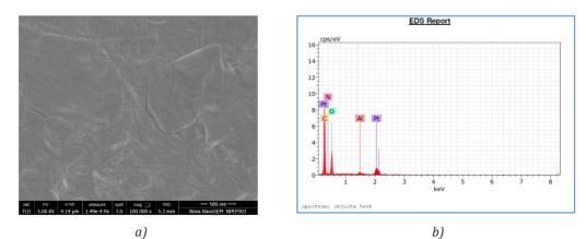
Figure 4: The LDPE surface: (a) SEM picture, and (b) EDS analysis results
