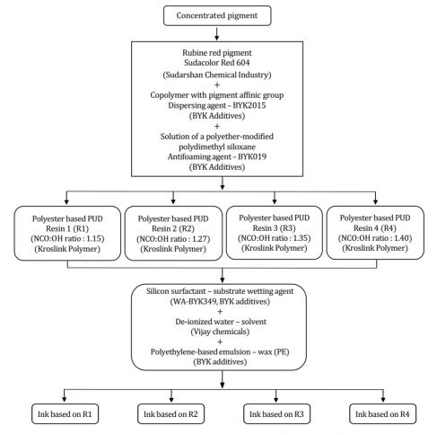
Figure 1: Flowchart for ink ingredients and stepwise addition
