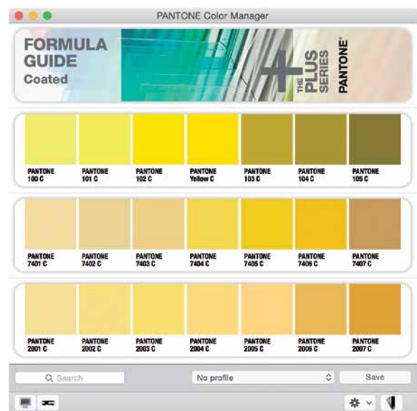
Figure 6: PANTONE Color Manager was used to extract and create a list of CIELAB values for the PANTONE + Solid Coated Library V2
