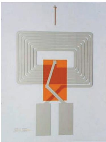
Figure 3: Printed moisture sensor with LC-circuit, dielectric, and wiring layers printed with ROKO printer at a speed of 1 m/min
