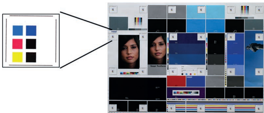
Figure 3: 63 \times 88 cm standard print test form with the 24 integrated measuring fields
