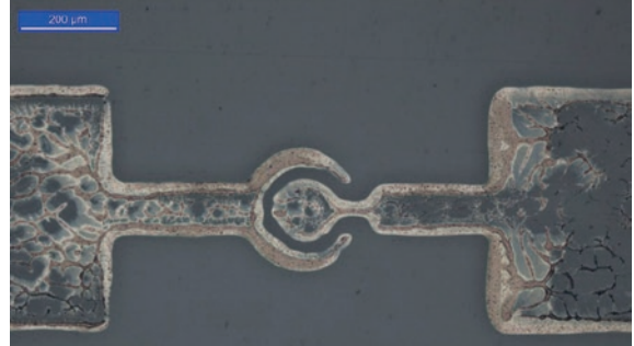
Figure 5: Typical seam or “halo” of a flexo printed pattern: the ink has been squeezed and has been deposited in the seam at the rim of the printed pattern; depositing ink within the intended areas has failed: only residuals of the ink have remained, and form a labyrinth-shaped structure
