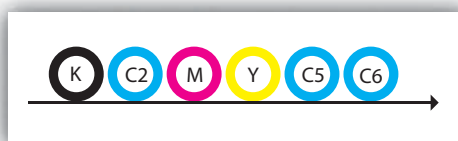
Figure 1: The ink sequence used during the printing trial
