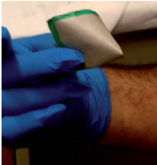
Figure 17: Self-supported unwound capacitor
