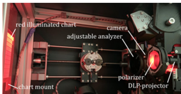
Figure 6: The capturing device with a mounted and red illuminated chart on the left and the DLP projector and M50 camera on the right
