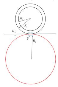
Figure 2: Model of contact of impression cylinders with the printing substrate in the gravure printing process  $(R_0$ - radius of the plate cylinder,  $R_1$  and  $R_2$ - radius of the impression cylinder with and without coating, H- thikness of printing substrate, S- zone of direct microcontact)
