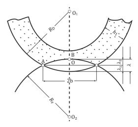
Figure 1: Scheme for calculating the pressure when printing by the gravure printing method where  $R_D$  is the radius of the impression cylinder,  $R_F$  is the radius of the plate cylinder and  $\lambda$  is the deformation
