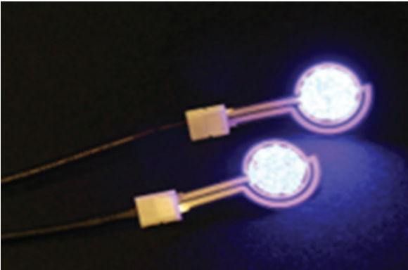
Figure 5: Printed micro-LED lamps
