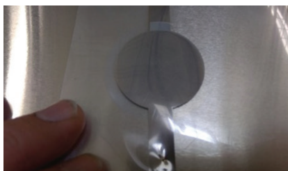
Figure 3: Large sample printed piezo-effect touch sensor
