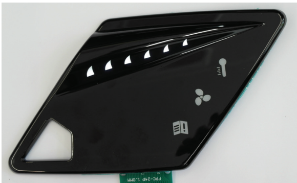
Figure 21: Final result of the injection moulding action
