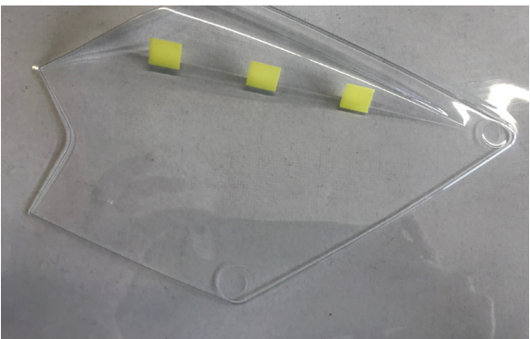
Figure 12: Test prints with phosphor layer after forming
