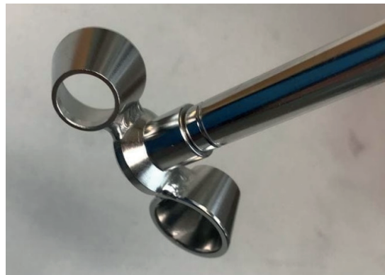
Figure 4: Cone shaped stirrer
