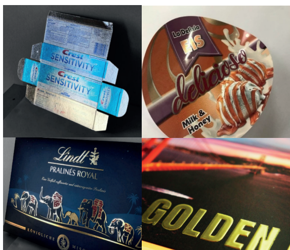
Figure 5: Samples metallized by foil fusing, cold foil transfer, hot foil stamping and digital hot foil stamping (sample from Konica Minolta) from left to right and up to down
