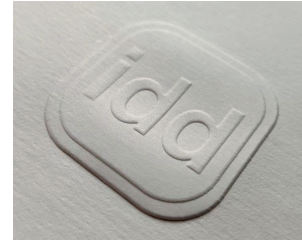
Figure 14: Embossing result in rough paper of 150 g/m 2 grammage by an additively manufactured embossing tool of 1 mm depth with a 0.1 mm tool gap, a force of 15 kN was applied to emboss the substrate; the embossment has a size of 38 mm × 38 mm
