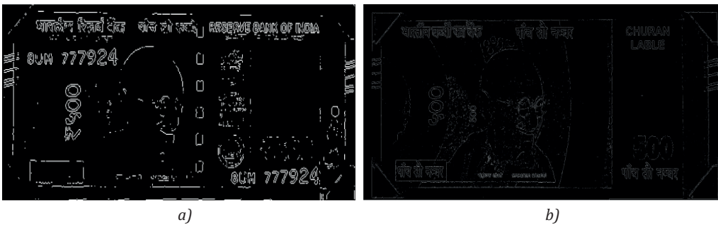
Figure 10: Sobel edge detection of real and dummy currency note: (a) real, and (b) dummy
