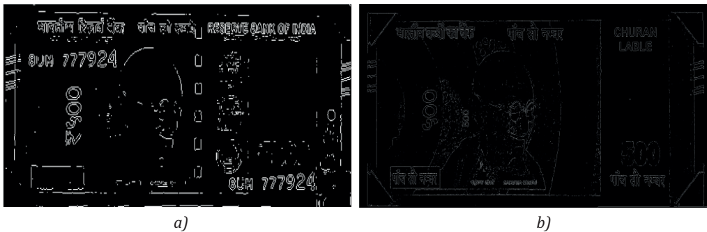
Figure 11: Prewitt edge detection of real and dummy currency note: (a) real, and (b) dummy
