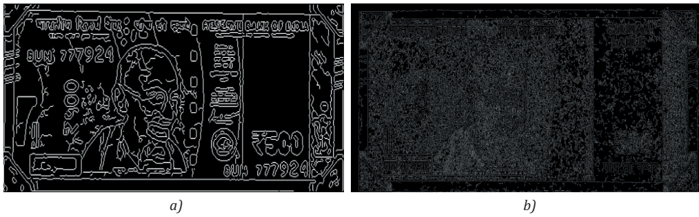
Figure 9: Canny edge detection of real and dummy currency note: (a) real, and (b) dummy
