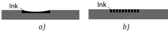
Figure 4: After the blading process the ink remains unsteady in the indentations without raster (a), with a raster the walls hold back the ink homogeneously (b)
