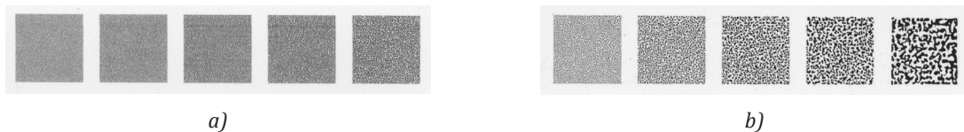
Figure 15: Printed charts B-04 (60–100 %) with PBK on primed surface (a) and on unprimed surface (b)
