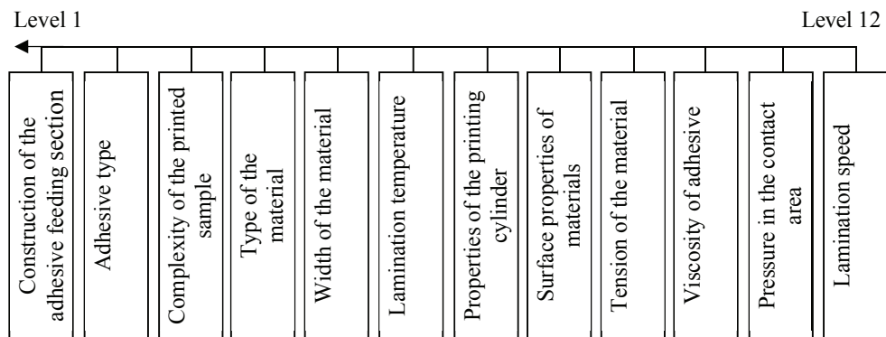
Figure 4: The model of the importance of quality factors of the solventless lamination process, as a result of the analysis of their relationships
