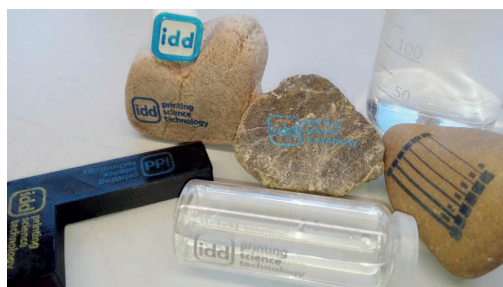
Figure 1: Examples of products printed with pad printing; photo from Hakimi Tehrani (2018)
