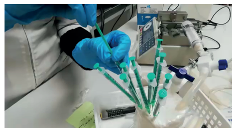
Figure 6: Taking care to isolate samples from contamination using a mechanical sealed pipette, transported in a film-sealed vessel
