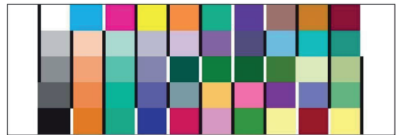
Figure 10: Custom test chart for the verification press runs showing the selected 27 test Pantone patches with tint ramps for black and three Pantone colors P151 C, Green C and P2091 C
