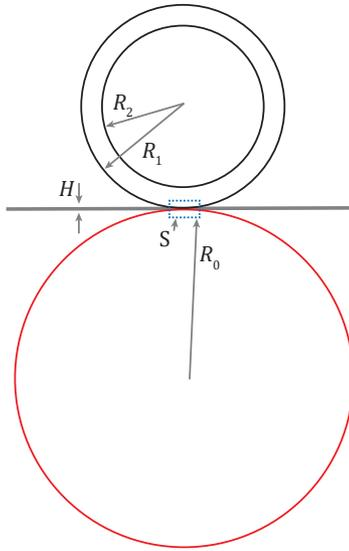
Figure 2: Model of contact of impression cylinders with the printing substrate in the gravure printing process ( $R_0$ - radius of the plate cylinder,  $R_1$  and  $R_2$  - radius of the impression cylinder with and without coating,  $H$  - thickness of printing substrate,  $S$  - zone of direct microcontact)
