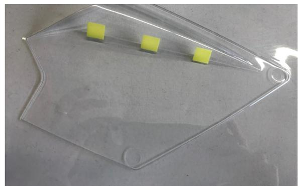
Figure 12: Test prints with phosphor layer after forming
