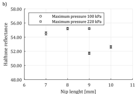
Figure 8: Halftone reflectance versus maximum pressure (a) and nip length (b)
