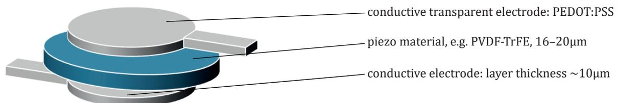
Figure 1: Schematic of the printed piezo-effect touch sensor
