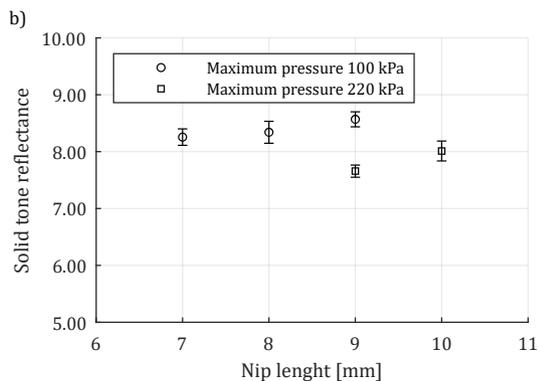
Figure 6: Solid tone reflectance versus maximum pressure (a) and nip length (b)
