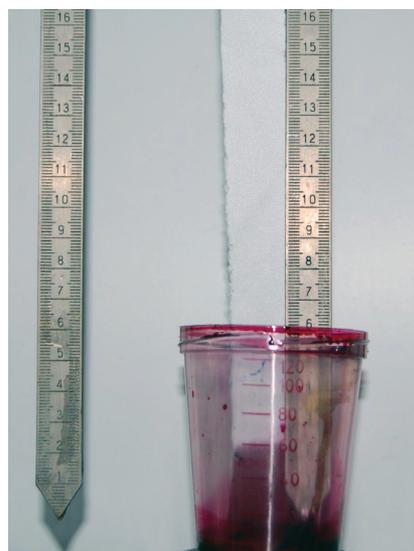
Figure 2: Klemm-type-capillary-rise method
