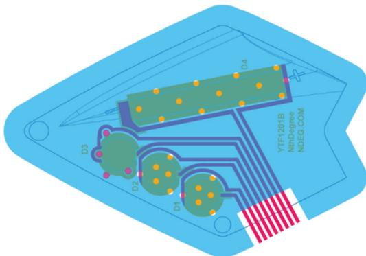
electrode: transparent conductive paste (NthDegree) – 140 mesh
