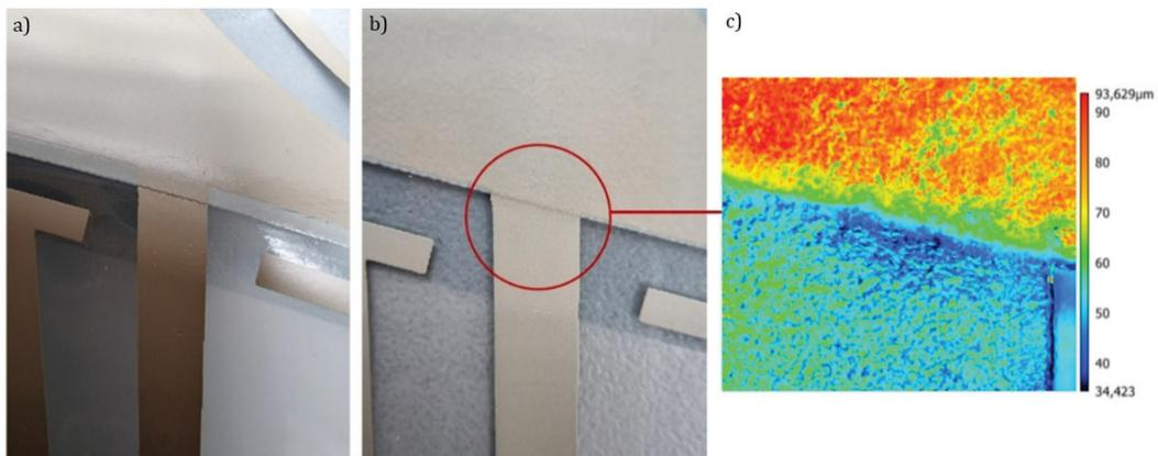
Figure 10: a) Crack after forming; b) enlarged before forming; c) height profile of the print before forming (ranging from 34.423 to 93.629 µm)
