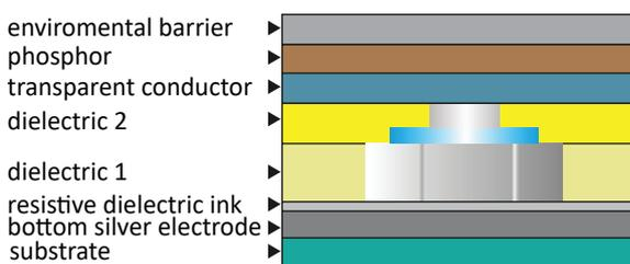
Figure 7: Sequence of printed layers with micro-LEDs (Claypole, 2019)
