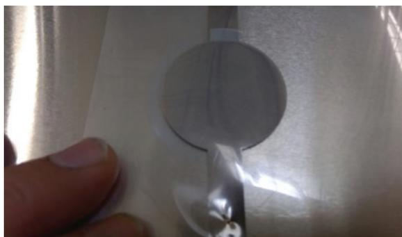
Figure 3: Large sample printed piezo-effect touch sensor
