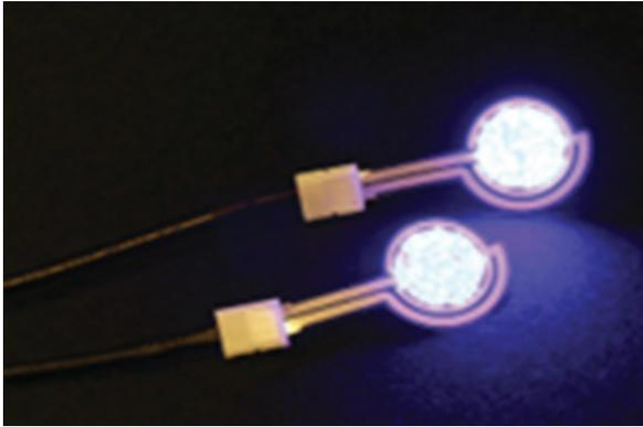
Figure 5: Printed micro-LED lamps
