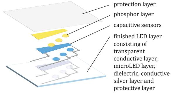
Figure 15: Adding capacitive switch and phosphor layer to the B-surface foil
