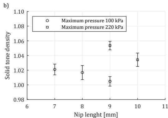
Figure 7: Solid tone density versus maximum pressure (a) and nip length (b)
