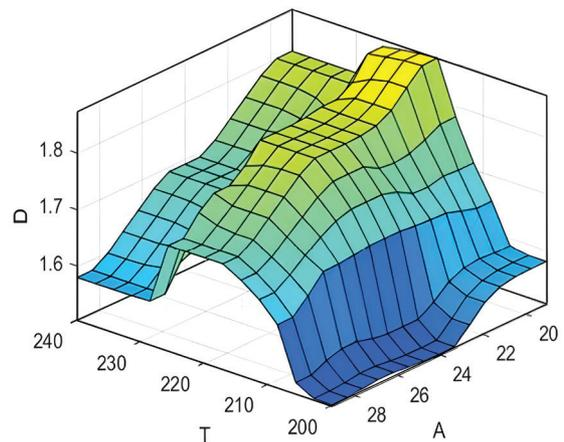
Figure 6: A model for forecasting the influence of the temperature and the absorption capacity on the optical density of a black ink layer
