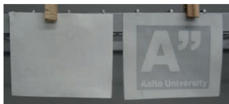
Figure 1: Wetting causes a visible opacity change in the hydrophilic areas; displayed here are two Aalto University logos printed with PS ink, shown dry (left) and after dipping in water (right)
